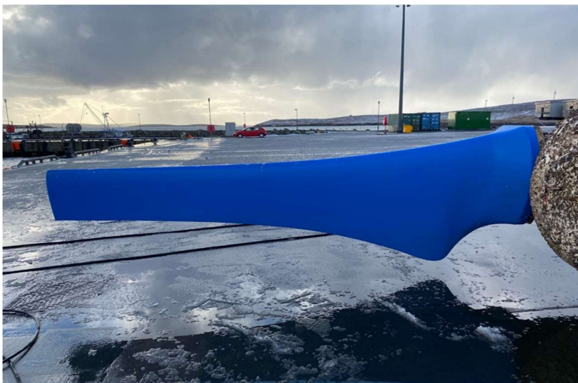
Figure 1: Negligible blade biofouling after 18 months of operation
