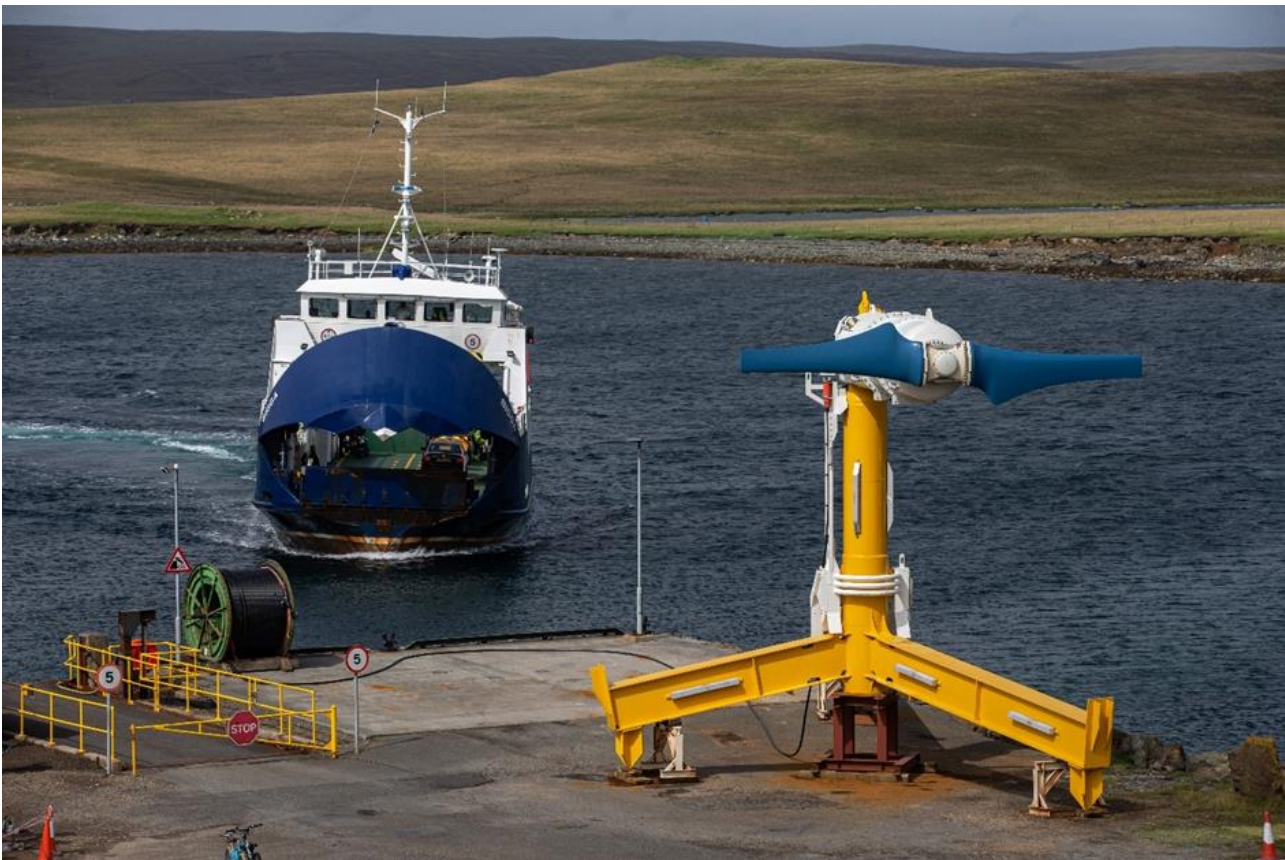
Figure 2-1 Nova Innovation's M100-D turbine quayside before deployment in Bluemull Sound, Shetland. Nova Innovation 2020 ©.
