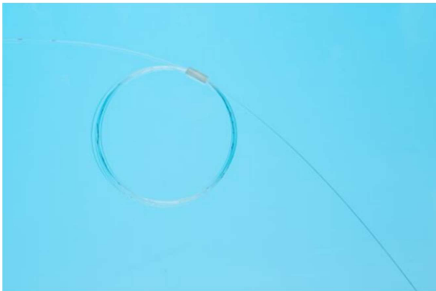
Figure 2 Smart Fibres FBG sensor (Smart Fibres, 2023)
