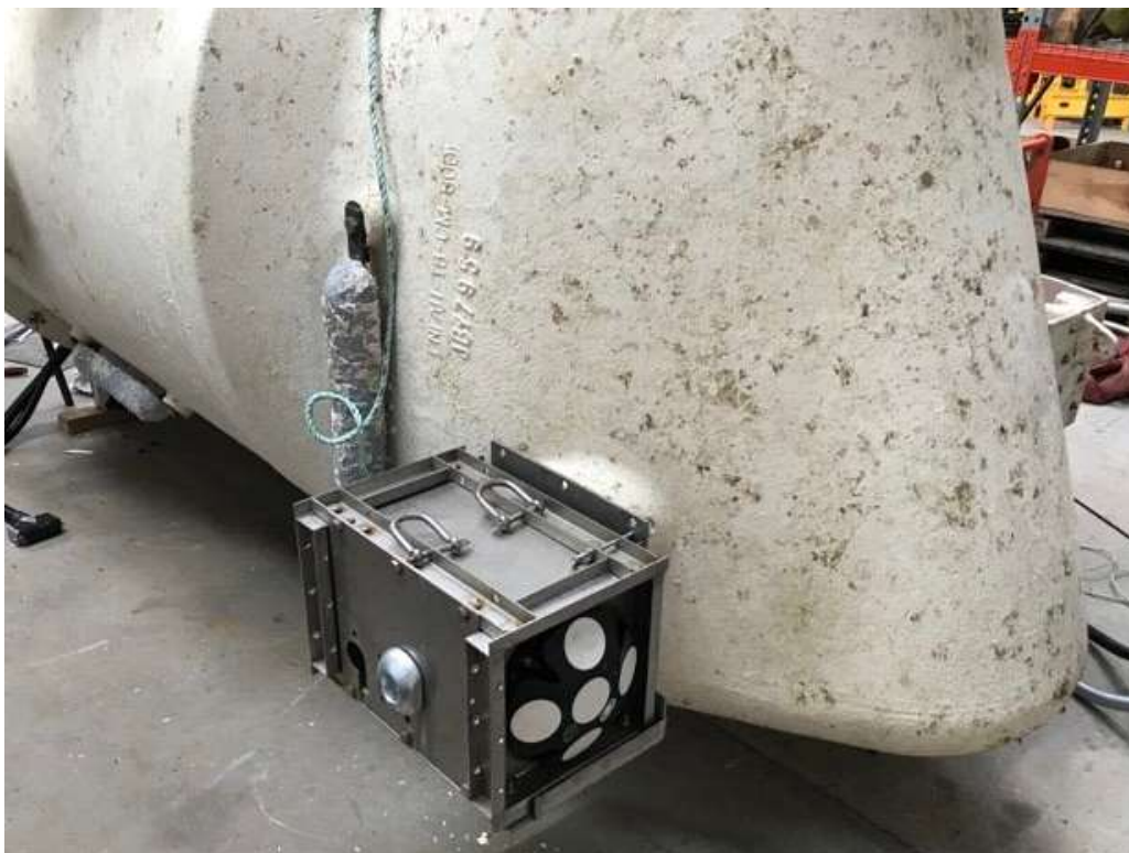
Figure 6 Nacelle ADCP mounted on rear of nacelle prior to deployment
