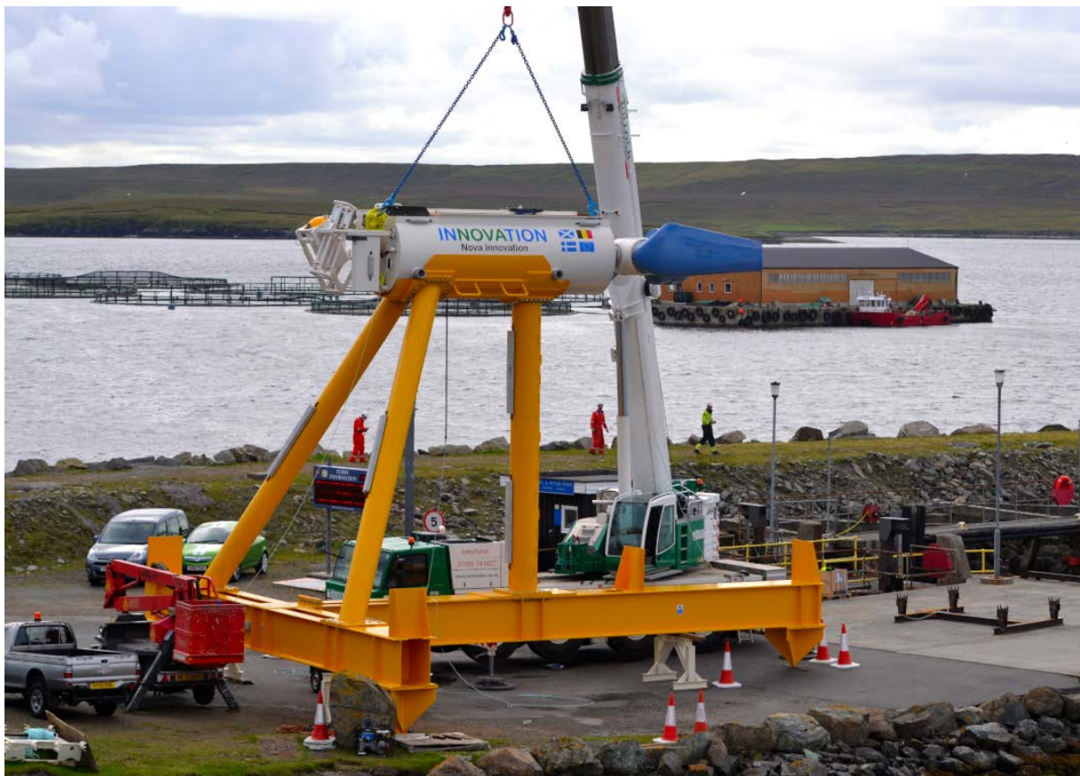
Figure 3.4. Nova Innovation M100 Tidal Turbine at Belmont, showing rotor blades in blue, cylindrical nacelle in white, and gravity base in orange.
