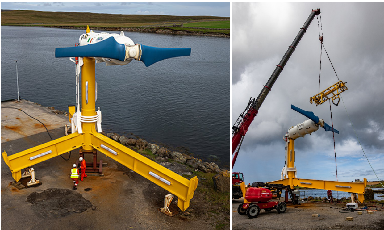
Figure 3.5. Nova Innovation M100-D Tidal Turbine, showing rotor in blue, cylindrical nacelle in white, and gravity base in orange. Lifting frame shown on right.
