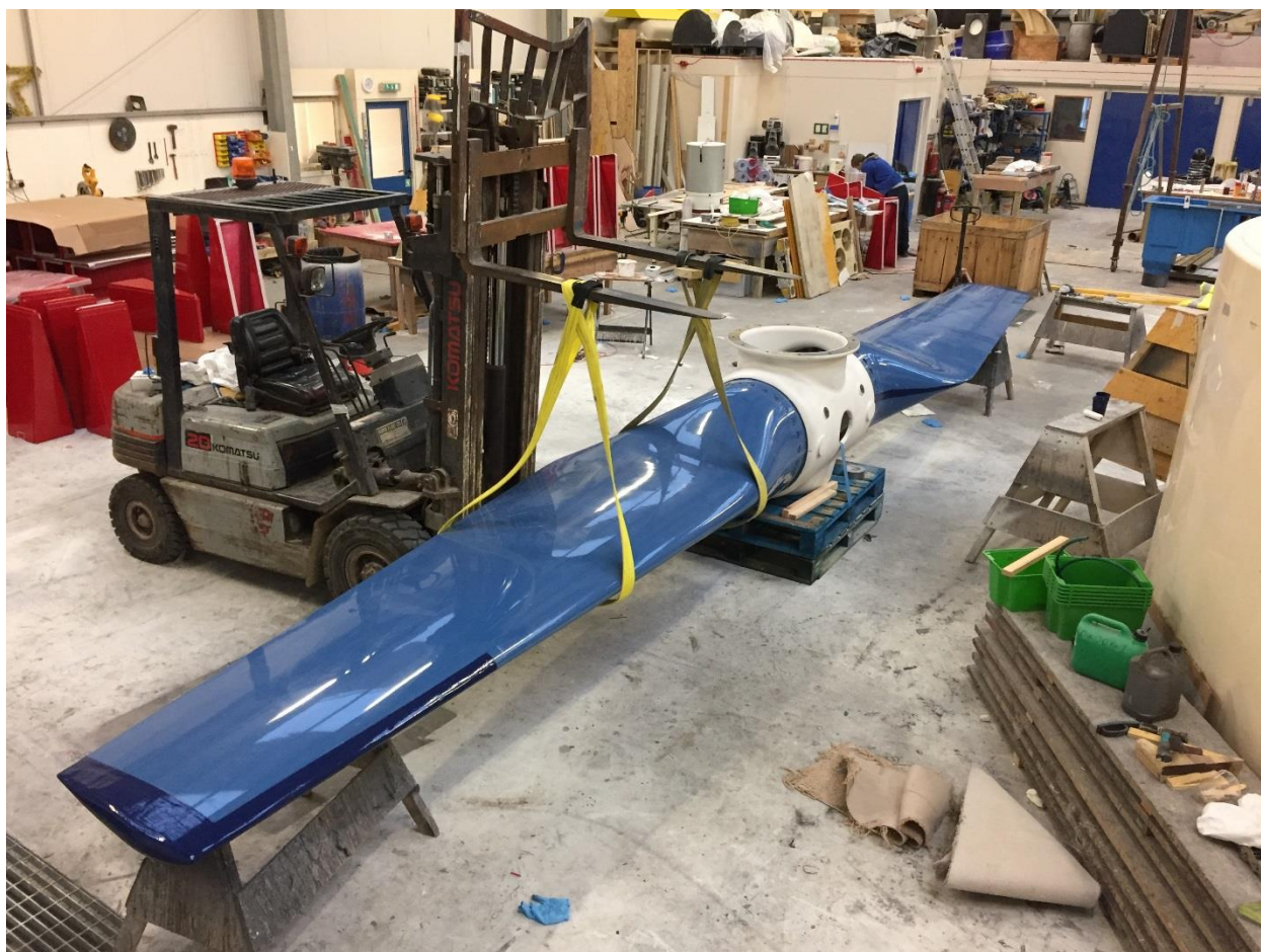
Figure 6.8. Shetland Composites manufacture of the turbine blades
