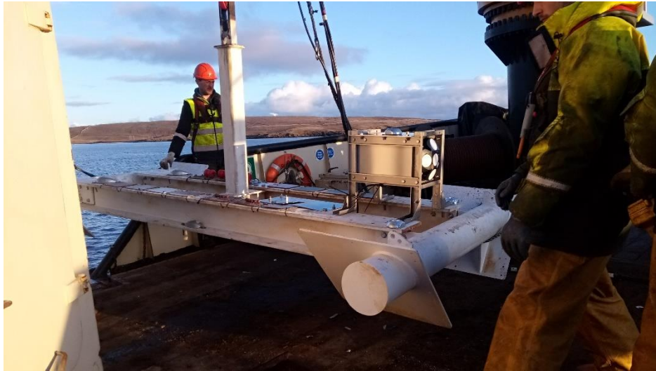
Figure 2.5: Instrumentation Skid Deployment
