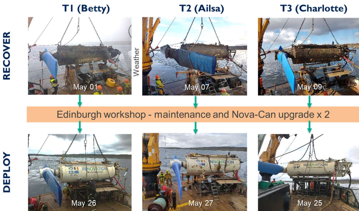
Figure 5-2: STA turbine recoveries and redeployments, May 2019
