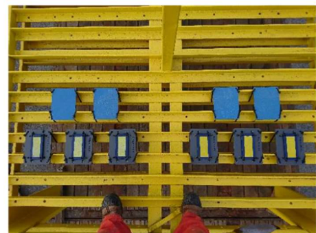
Figure 8-8: M100 turbine blades after >1 year of operations; biofouling test pieces
