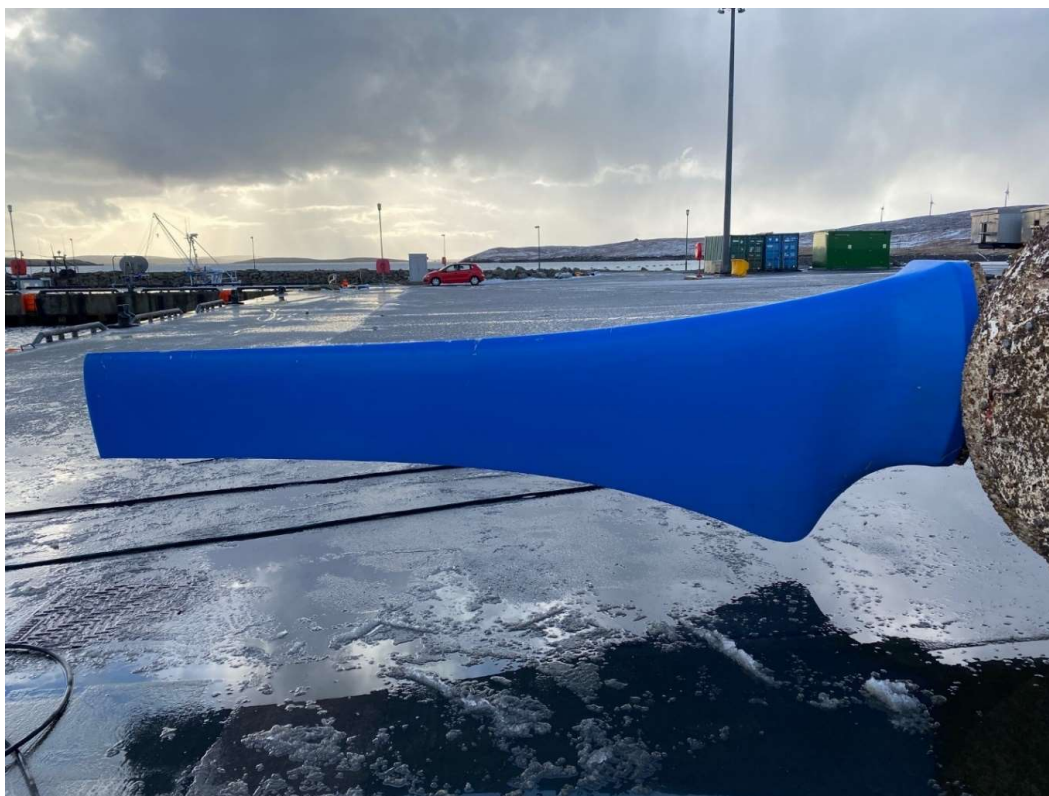
Figure 8-9: Negligible marine growth on T4 rotor after 24 months of operation
