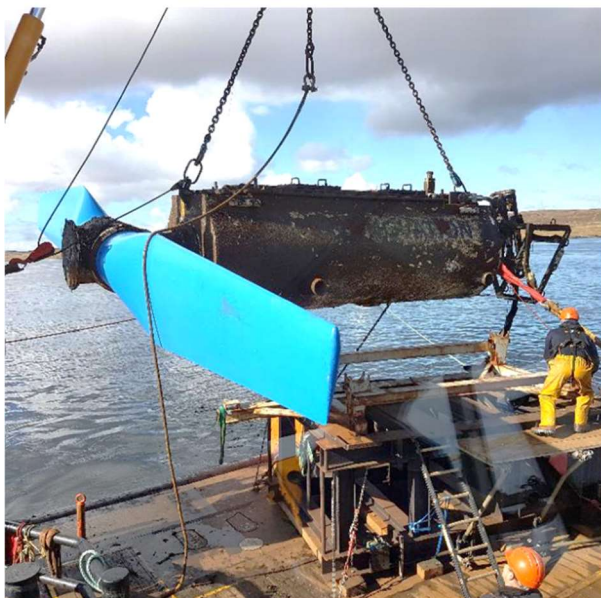
Figure 8-8: M100 turbine blades after >1 year of operations; biofouling test pieces
