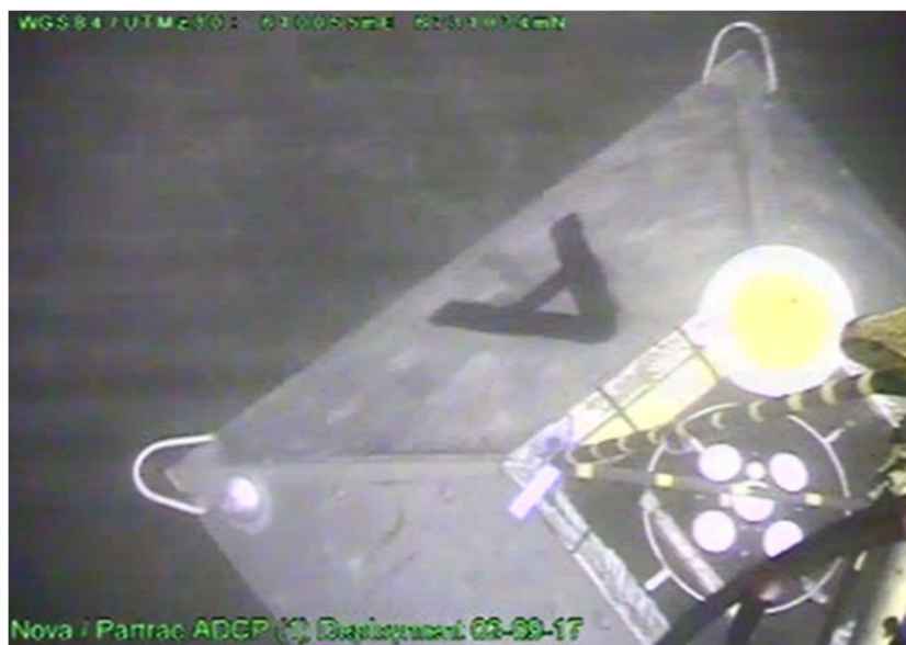
Figure 6-3: Seabed mounted ADCP instrumentation deployment
