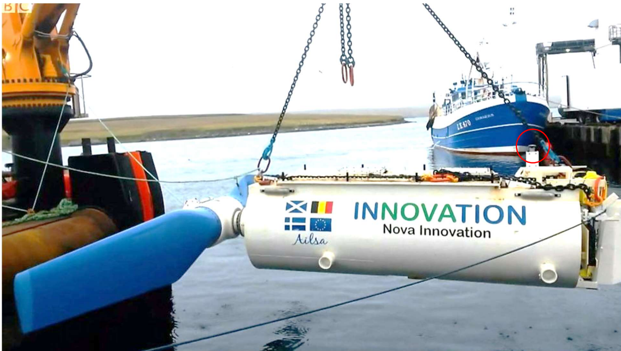
Figure 4-1: Nova M100 turbine showing position of flow sensor (red circle)
