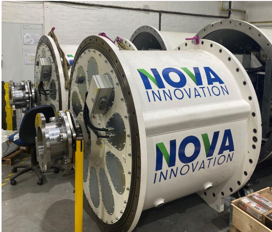
Figure 4: The generator module at Nova's Manufacturing Facility, Edinburgh, during the final assembly process
