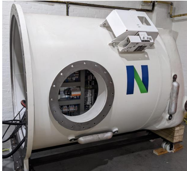
Figure 5 - Fully assembled ECM, prior to full turbine assembly
