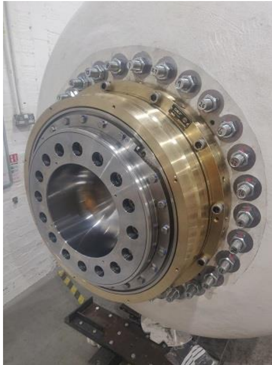
Figure 3: The new main shaft sealing solution implemented on T6
