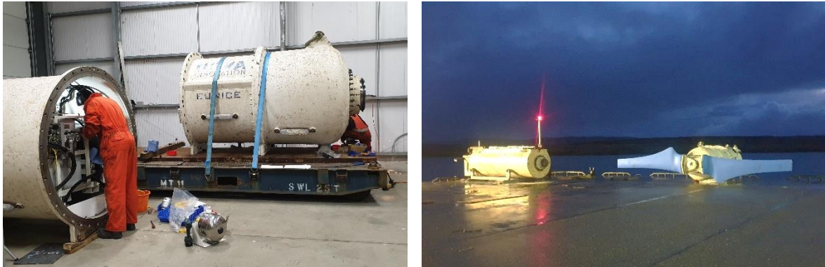
Figure 7: T4 local maintenance; M100 nacelle and T4 ready for redeployment
