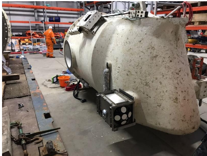
Figure 10: Nacelle-mounted ADCP on turbine T4
