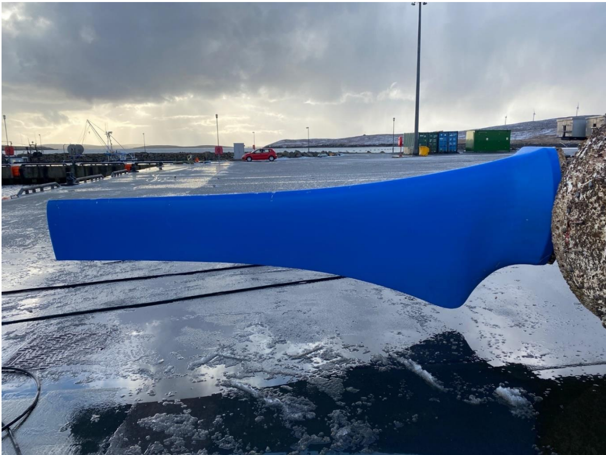
Figure 14: Negligible marine growth on T4 rotor after 18 months of operations
