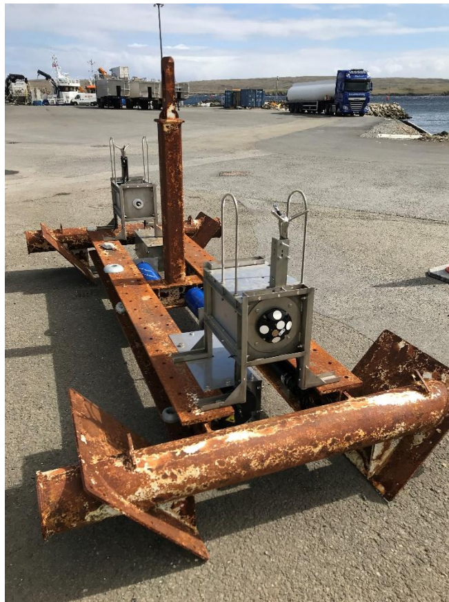
Figure 10: Instrumentation skid with ADCP and ADV mounted
